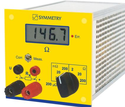
Mikroommetar domaćaja  $200 \mu\Omega$  do  $20 \Omega$ , SM216.
